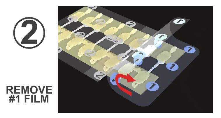
Remove #1 release paper and do not remove #2 release paper at this step
